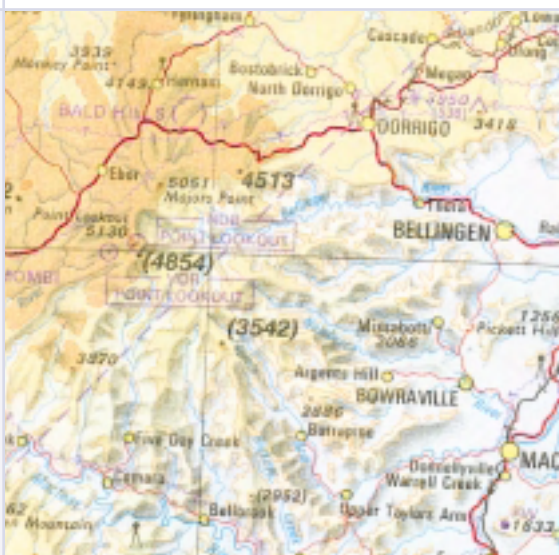
Example of hypsometric tinting. Source: Armidale World Aeronautical Chart.
